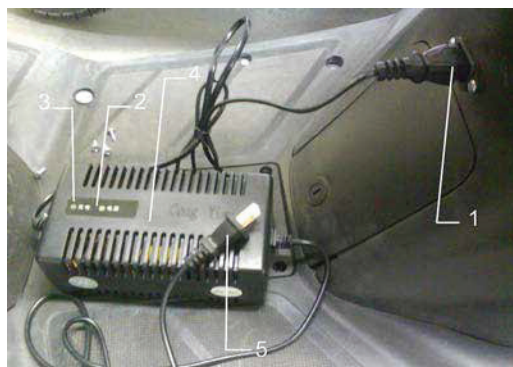
1. Plug (to scooter) 2. Indicator 3. Charge Indicator 4. Charger 5. Plug (to outlet)
